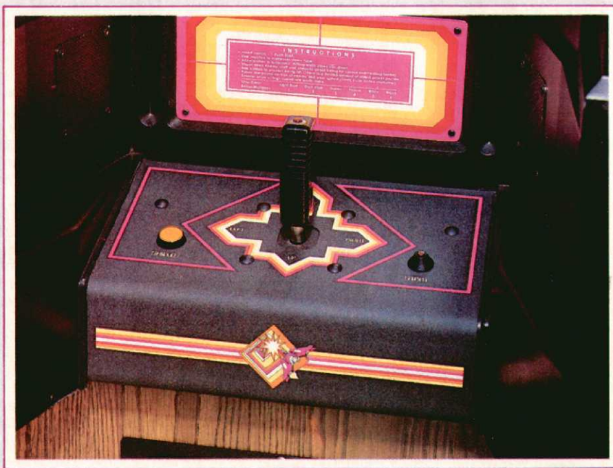
A standard top-firing joystick as seen on the control console from Centuri's Tunnel Hunt
